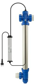
The housing is made of DUPLEX stainless steel and comes with Ø63mm to Ø50mm fittings and  $1\frac{1}{2}$ " female threaded inserts.
