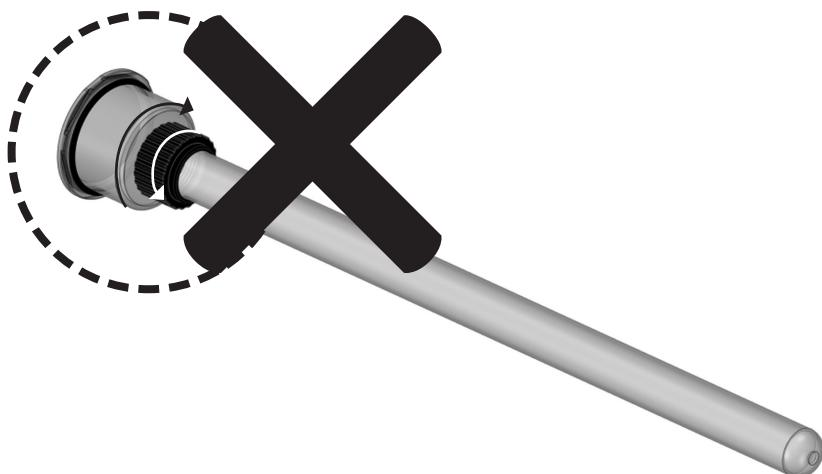
**EN: Do not disassemble!** The quartz glass connection cannot and may not be dismantled.
