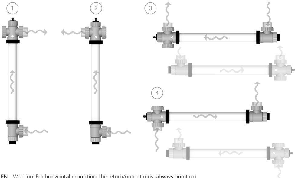
EN Warning! For **horizontal mounting**, the return/output must **always point up**.
